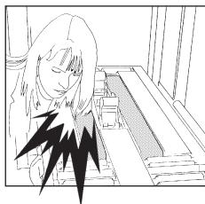
**WARNING!** Cavity in the conveyor bed.
