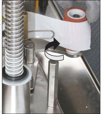
Put a box inside of the machine and adjust the lateral guide and adjust the hieght positon of unit tape and put on the top head with drive belts.
