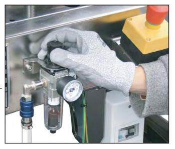
If necessary rotate the nozzle to optimize the air flow.
