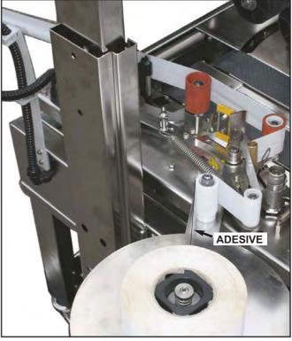
Correct path and positioninf the tape flap on robber roll. Repite this operation on the other unit tape.
