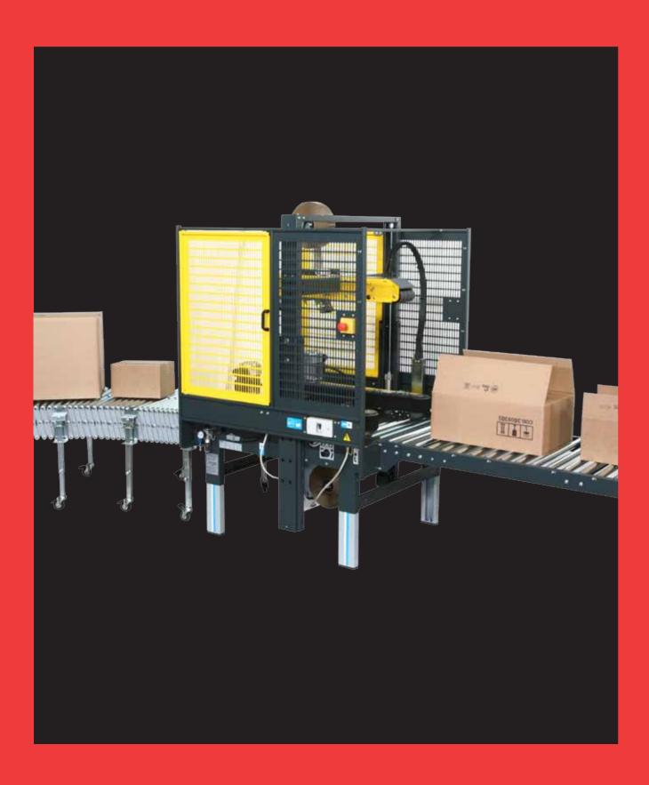
Side drive, semi-automatic random carton sealing machine for large cartons.
