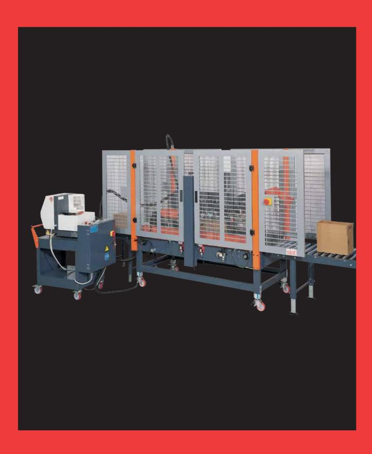
Fixed size, manually adjustable, side drive, hot-melt carton sealer with flap folder.
