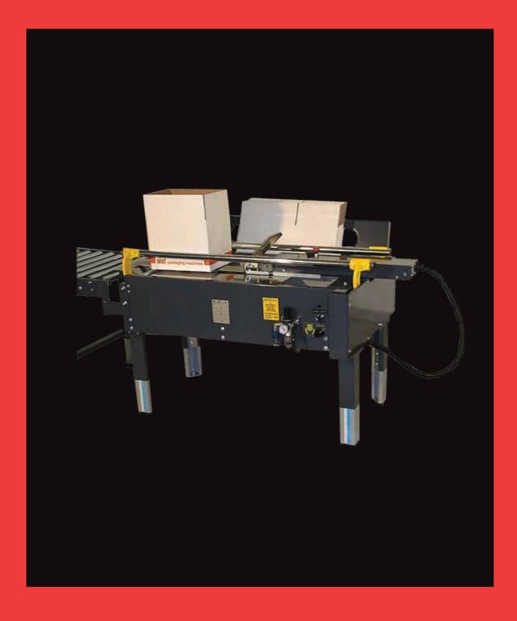
Semi-automatic carton erector and manual filling station with box pusher.
