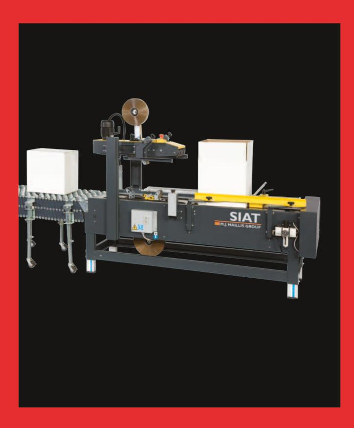
Semi-automatic box filling/erecting/ sealing packaging station, manual set up according to the different carton sizes for forming, manual filling and sealing of the top/bottom of the carton.
