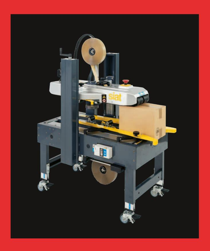
Fixed size, manually adjustable top and bottom drive carton sealing machine.
