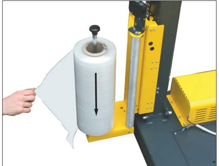
Secure the film to the pallet as shown in the figure.
