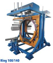
Horizontal automatic stretch wrapping machine for medium size products.
