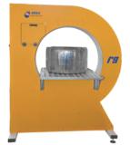
Semi-automatic machine for packaging of car tyres, single or up to four stacked - complete with ball transfer tables - start-stop ring by foot pedal, automatic clamping/cutting film unit and manual positioning of the product inside the machine.
