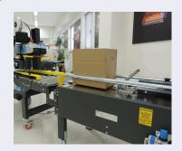
According to the different semiauto case sealer in SIAT range, dedicated fixing plates are available to integrate F105 to create a complete packing station
