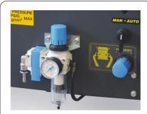
With a selector it is possible to work in both manual and automatic operations increasing the speed performance
