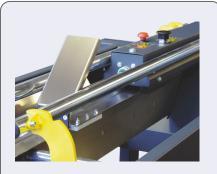
Easy and safe bottom flap folding system combined with tubolar pneumatic centering system, that holds the boxes in vertical to proceed with product filling and final sealing
