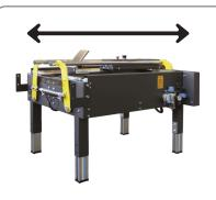
In case of need for processing longer boxes, a special "Long" version of F105 is available to cover up to 800mm.
